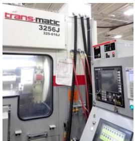
F instrument. Trans-Matic is currently testing small volume cylindrical stamped parts on a press with a 30pa leak rate reject limit (approximately 30sccm), at 5 psi test pressure with a total leak test cycle time of .14 seconds.
