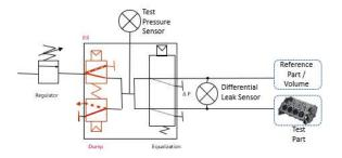
Uses two pressure sensors, one to measure the test pressure and a second to measure the differential pressure drop from a leak. The pressure is equalized on both sides of the differential pressure sensor during the fill and stabilize steps. The test step isolates the test from reference to measure the leak as a differential pressure drop over time multiplied by the parts volume.
