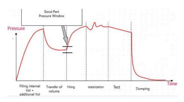
The volume test itself has to be very accurate and repeatable. On this system, the test is based on PV=nRT, known as Boyle-Mariotte 's Law.
