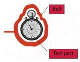
Watch manufacturing is not perfect. Production watches will have volume variations. These volume variations prevent the test chamber from being of a design that is too tight, and they also create a variability in the initial volume test.
