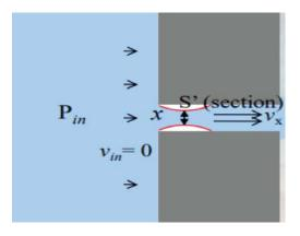
This reduced diameter path is called a "vena contracta" which, on sharp angle cylindrical path, typically reduces the apparent diameter of the hole by 15% to 25%.
